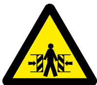
Risk of crushing
